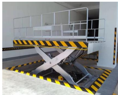
Scissor lift (Lever, screw, rack gear)
